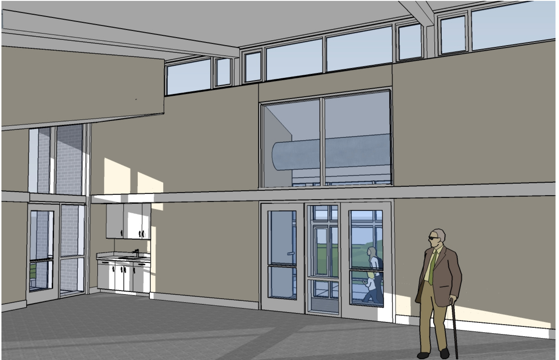
5. Interior View Multi-Purpose Room Looking N : Beyond this main entrance to the Multi-Purpose Room are the stairs down to the Gallery, with the porch and lawn beyond. At the top is the row of clerestory windows for enhanced daylighting. In the corner to the left is the convenience sink and cupboards for functions in this room. The doorway on the left is for exit in the event of fire; it leads to a balcony with steps connecting to the playground stairway.
